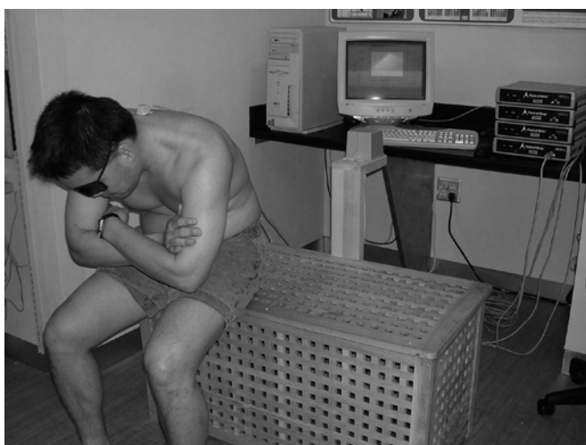
FIGURE 1. Subject performing forward flexion trunk repositioning sense task. A Flock of Birds sensor is attached over the T1 vertebra, the electromagnetic source is mounted on a wooden bracket in the middle of the seat, and the Flock of Birds system is on the right side of the work shelf.
